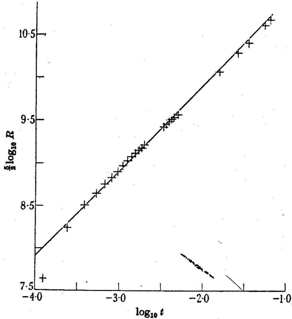
FIGURE 1. Logarithmic plot showing that  $R^{\frac{1}{2}}$  is proportional to  $t$ .
