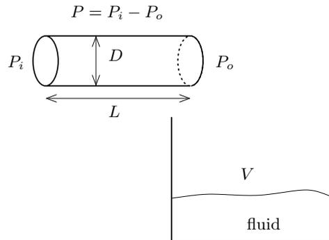
The time required to fill in the vessel depends directly on the flow coming out of the pipe. The flow depends on the diameter of the pipe ( $D$ ) and on the velocity of the liquid. The driving force in this experiment is the pressure (we assume gravity is not involved) which act through its gradient. Therefore  $P = P_i - P_o$  and  $L$  must be considered as relevant variables. The viscosity  $\mu$
