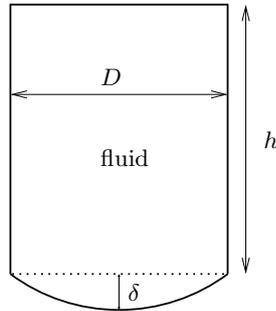
The relevant physical quantities in this problem are the geometry of the vessel (parametrized by  $d, D$  and  $\delta$ ), the density  $\rho$  and the height  $h$  of the liquid which determine the action of the gravity and the modulus of elasticity  $E$  which gives a relation between stress and deformation (it relates somehow the pressure and  $\delta$ ).
